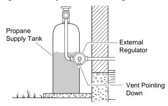
Figure 12 - External Regulator With Vent Pointing Down
